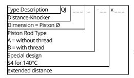
For Example: Distance-Knocker Type QJ100 Piston Rod without thread Special design up to 140°C Extended distance 150 mm Part Number: QJ100A-S4X150
