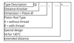
For Example: Distance-Knocker Type QJ100 Piston Rod without thread Special design up to 140°C Extended distance 150 mm Part Number: QI100A-S4X150
